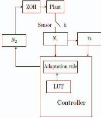
Figure 2: Schematic Block Diagram of Adaptive Regulator
