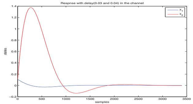
Figure 6: State values of the double integrator system with network loading using True Time simulation
