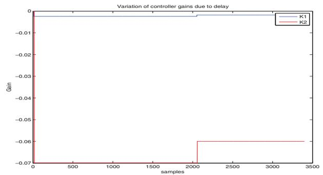
Figure 7: Variations in controller gains in True Time simulation
